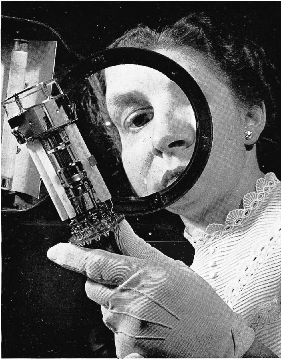
FIG. 6. Operator examining the three-gun assembly during fabrication of the RCA-21AXP22 Color Kinescope at the RCA Tube Division plant, Lancaster, Pa. The three guns are converged mechanically and magnetically and are focused electrostatically. Provisions are made for individual adjustment of each beam radially, and the blue gun beam may be adjusted laterally as well. This design permits dynamic convergence during the scanning of the tube.
