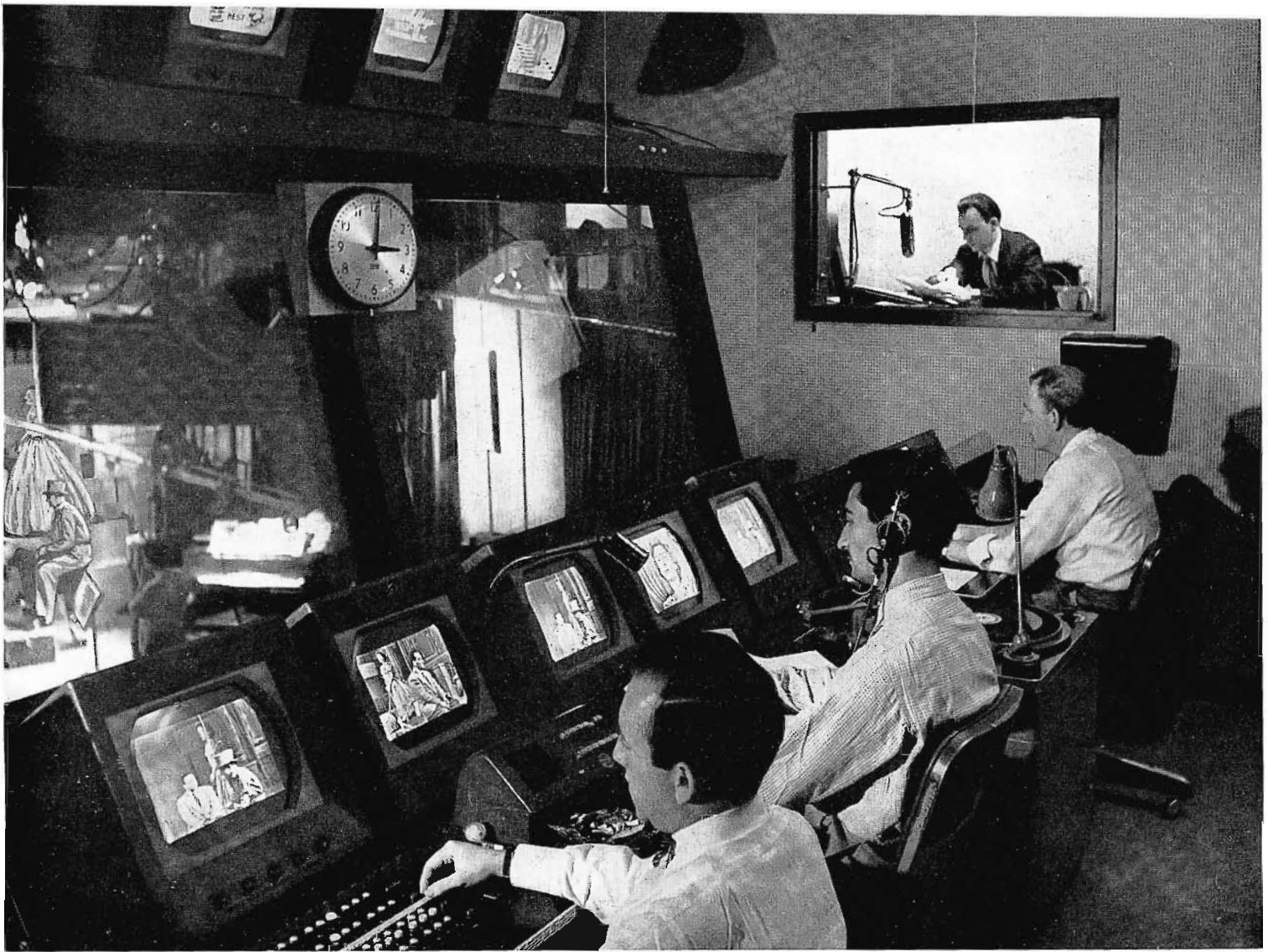
FIG. 14. Studio 11 control room in action. Left to right are video switcher, director, audioman and announcer. Camera control operator sits farther to left (not shown).
